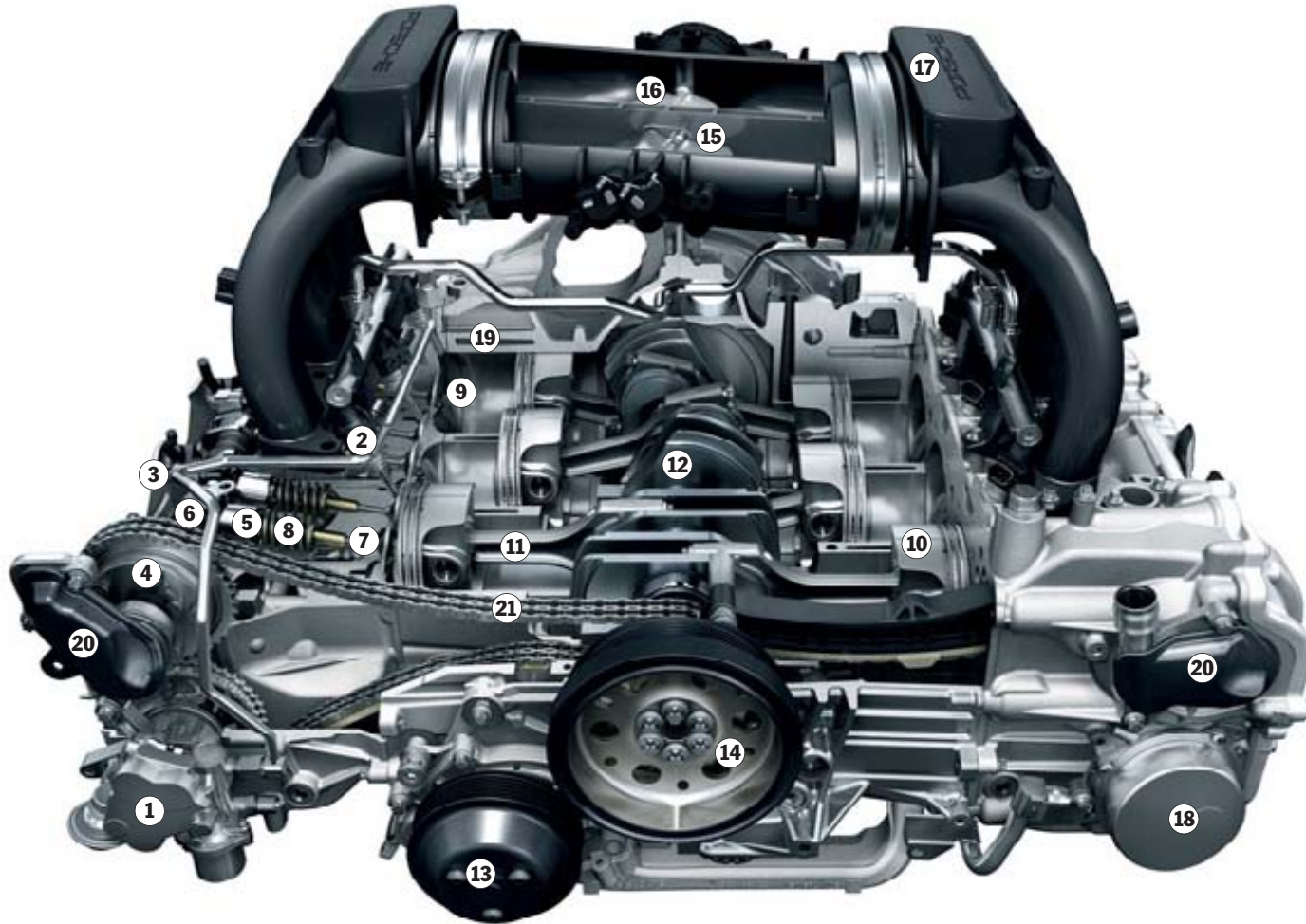
3.4-litre six-cylinder Boxer engine in the Boxster S
