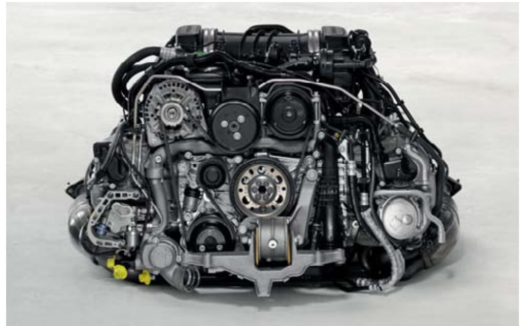
3.4-litre six-cylinder Boxer engine in the Boxster S
