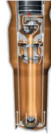
Rebound in 'Normal' mode – working piston and bypass, sporty-comfortable tuning
