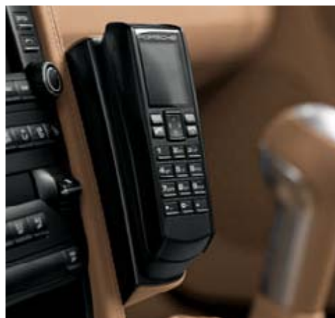
Cordless handset for telephone module and PCM
